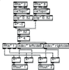
Fig. 21. The pfft~ subpatch used to multiply the spatial pattern of a stereo signal on to a monophonic signal. (Lippe & Torchia, 2003).
