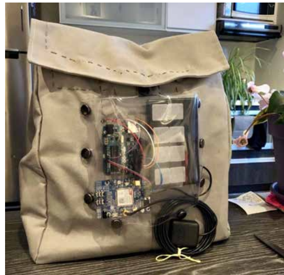
Figure 1. La Encomienda closed with the electrical-electronic digital components; the artifact works through a circuit done with conductive thread that activates the sending of the message once the bag is unbuttoned.
